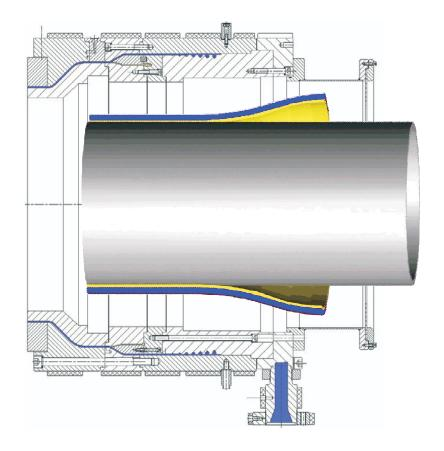
This two-layer die is used for coating pipes up to 700 mm diameter with intermediate adhesive layer.
