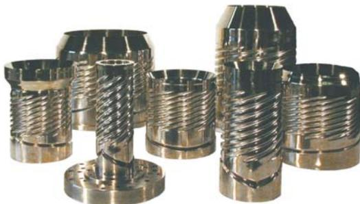
Spiral mandrel manifolds for a 7-layer blow moulding die head for filler pipes
