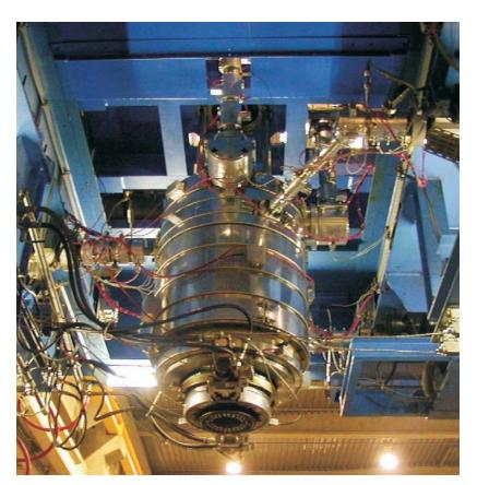
ETA 6-layer die head in a modified blow moulding machine
