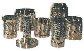
Spiral mandrel manifolds for a 7-layer blow moulding die head for filler pipes
