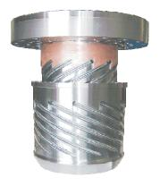
ETA coextrusion die heads with 6 or 7 layers are a very favourable proven solution for the blow moulding of multi-layer plastic fuel tanks and multi-layer filler pipes for automotive applications. Also and increasingly, 2 and 3-layer die heads are supplied for industrial containers, e. g. drums and IBC.
